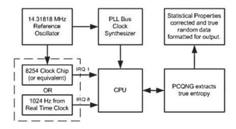
The fundamental source of entropy in the PCQNG is the same as in virtually all types of TRNG devices. These devices consist of two distinct parts: one is a fluctuating signal source having an unpredictable temporal evolution; the second is a periodic signal, causally independent of the first signal, that is used to generate a timing sequence for sampling the first signal.
